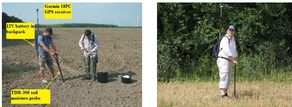
Figure 6 Construction and application of the Spectrum TDR-300 soil moisture measuring device
