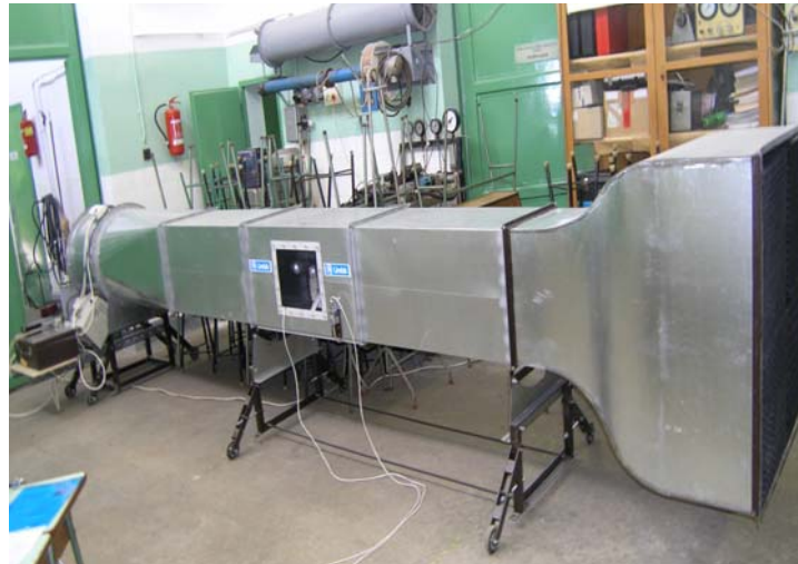
Fig. 2.2 Wind tunnel in the laboratory of FME SZIU (designer: F. Szlivka – B. Balló) (source: author's photograph)
