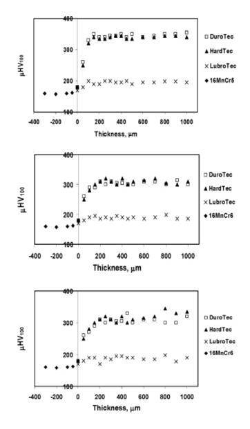
Figure 2. In-depth distribution of microhardness, SOD from top to bottom 180 mm, 100 mm, 260 mm
