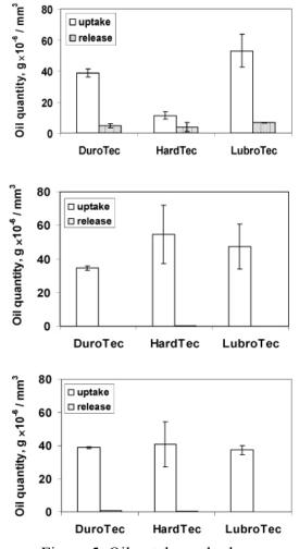
Figure 5. Oil uptake and release SOD from top to bottom 180 mm, 100 mm, 260 mm
