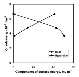
Figure 6. Oil release on the components of surface energy
