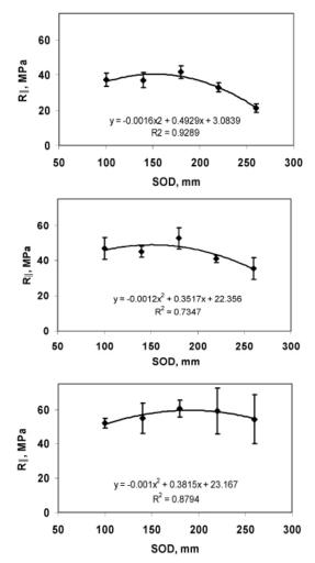
Figure 4. Shear component of coating bond strength, R<sub>∥</sub> From top to bottom: DuroTec, HardTec, LubroTec
