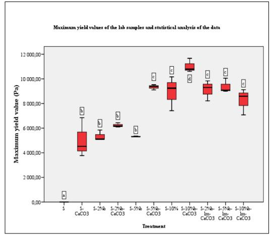
Figure 2: Maximum yield values of the flow curves of laboratory samples, significant differences are indicated with the small letters of the ABC, with a confidence interval of 95%
