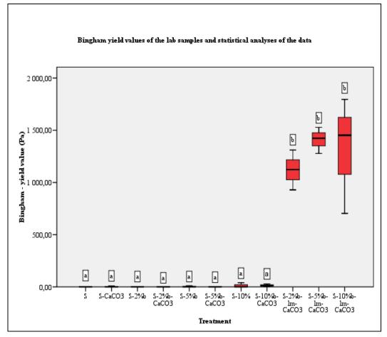
Figure 3: Bingham –yield values of the flow curves of laboratory samples, significant differences are indicated with the small letters of the ABC, with a confidence interval of 95%
