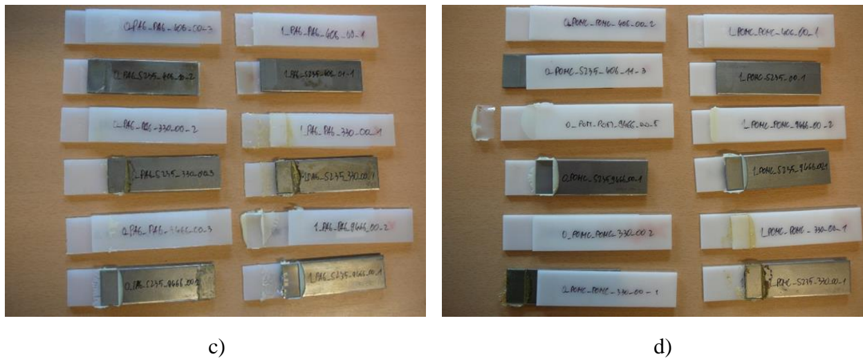
Fig. 4.16. Different failure types of different joints after lap-shear testing: a) PEEK, b) PET, c) PA6-E, and d) POM-C, (untreated to the left, treated to the right)
