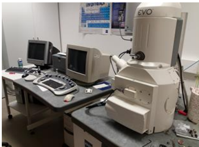
Fig. 3.14. Scanning electron microscope SEM which used to scan polymer surfaces morphology
