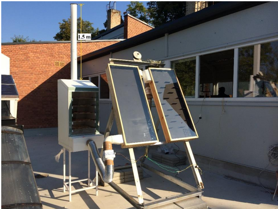
Fig. 3.21. Solar drying system illustration in laboratory
