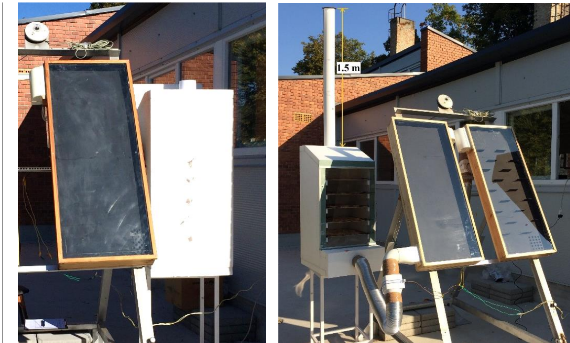
Fig. 4.49. Solar drying system with and without chimney integration
