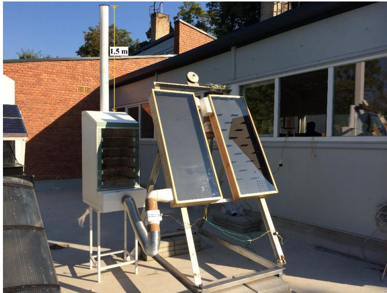
Fig. 6. Solar drying system illustration in laboratory
