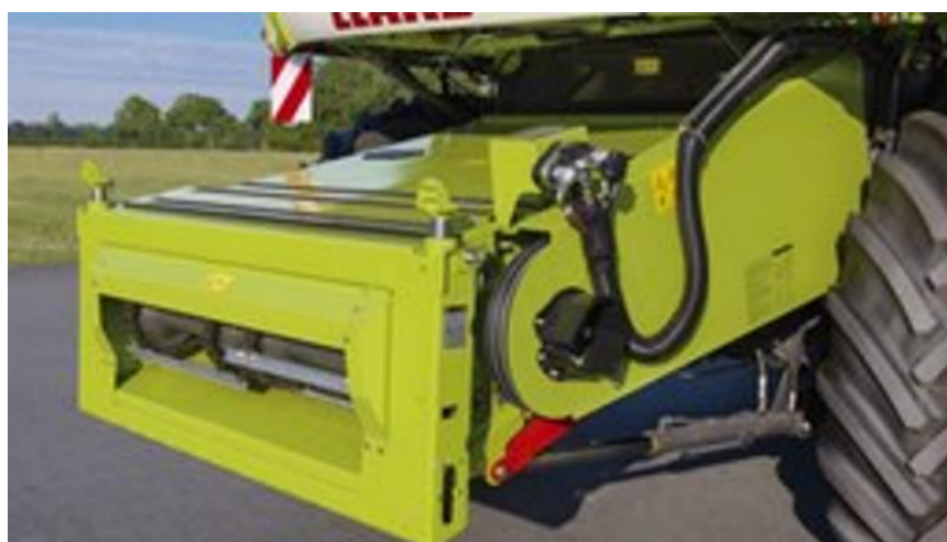
Fig. 3.9. CLAAS combine harvester feeding house
