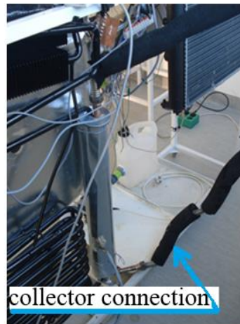
Fig. 6. Absorption cooler connected with solar collector
