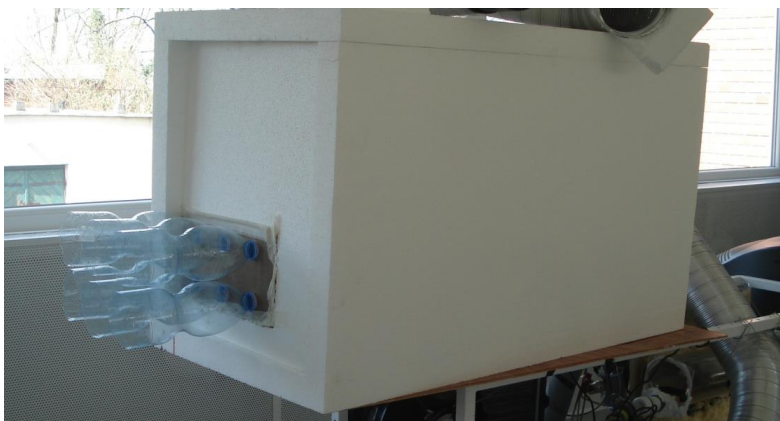
Fig. 4. Experimental alternative cooler with bottles
