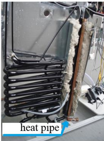
Fig. 6. Absorption cooler connected with solar collector
